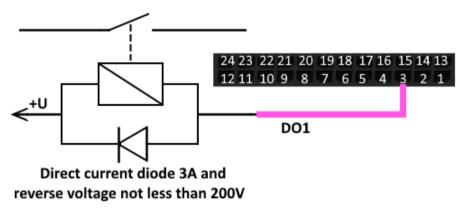
By default, after a device reboot, the state of the digital output is reset to 0, that is, "off". In the settings, it is possible to save the state of the device output and digital outputs of the connected <u>extension</u> <u>unit</u>.
